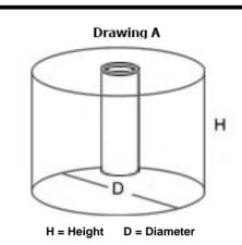
Size of PVC sleeve provided: 20-ft pole: ID = 6"ID / Length = 24" 25-ft pole: ID = 6"ID / Length = 30" 30-ft pole: ID = 6"ID / Length = 36" 35-ft pole: ID = 6"ID / Length = 42" 40-ft pole: ID = 6"ID / Length = 48"
