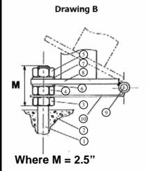
1 Threaded anchor rods M20 2 Concrete 300kg 3/4/5 Nuts M20 6/7 Washers M20
